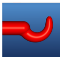
Optimale Anguss-Geometrie, gut verrundet Optimum gate geometry, with edges rounded
