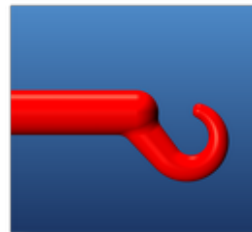
Optimale Anguss-Geometrie, gut verrundet Optimum gate geometry, with edges rounded
