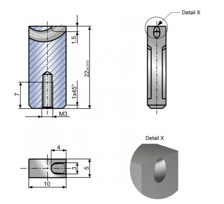
For tunnel gating of small, thin-walled moldings. This gate insert has a closed gate diameter and is therefore suitable for the use of low article weight and for very thin-walled moldings.
